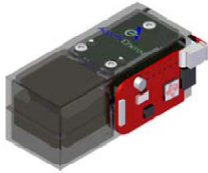
Figure 1. JTRA-e5mini in “kit” form, shown with a Texas Instruments eZ430-CC2500 wireless microcontroller board solely powered by the AdaptivEnergy harvester.
